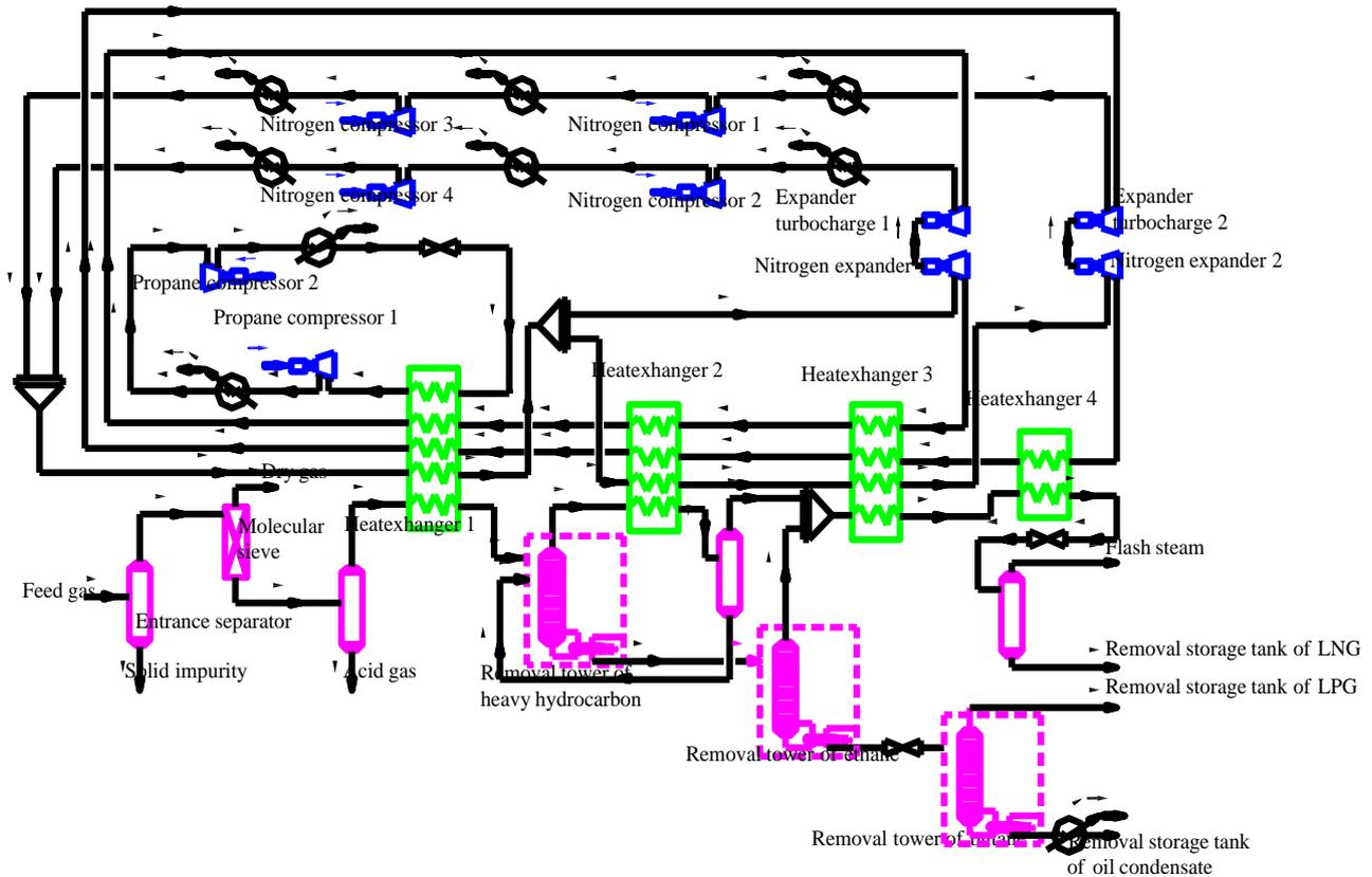
FIGURE 2 Flow chart of liquefaction process with propane precooling device and double nitrogen expander
