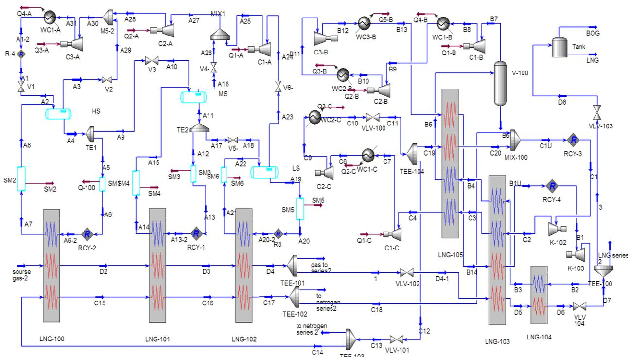
FIGURE 3 Schematic of HYSYS simulation of FLNG liquefaction process
